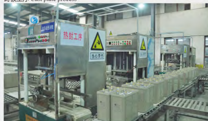
热封工序 Heat sealing process
