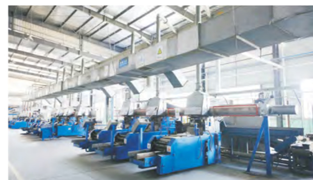
铸板工序 Slab casting process
